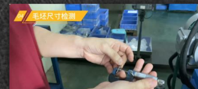
Roughcast size inspection
