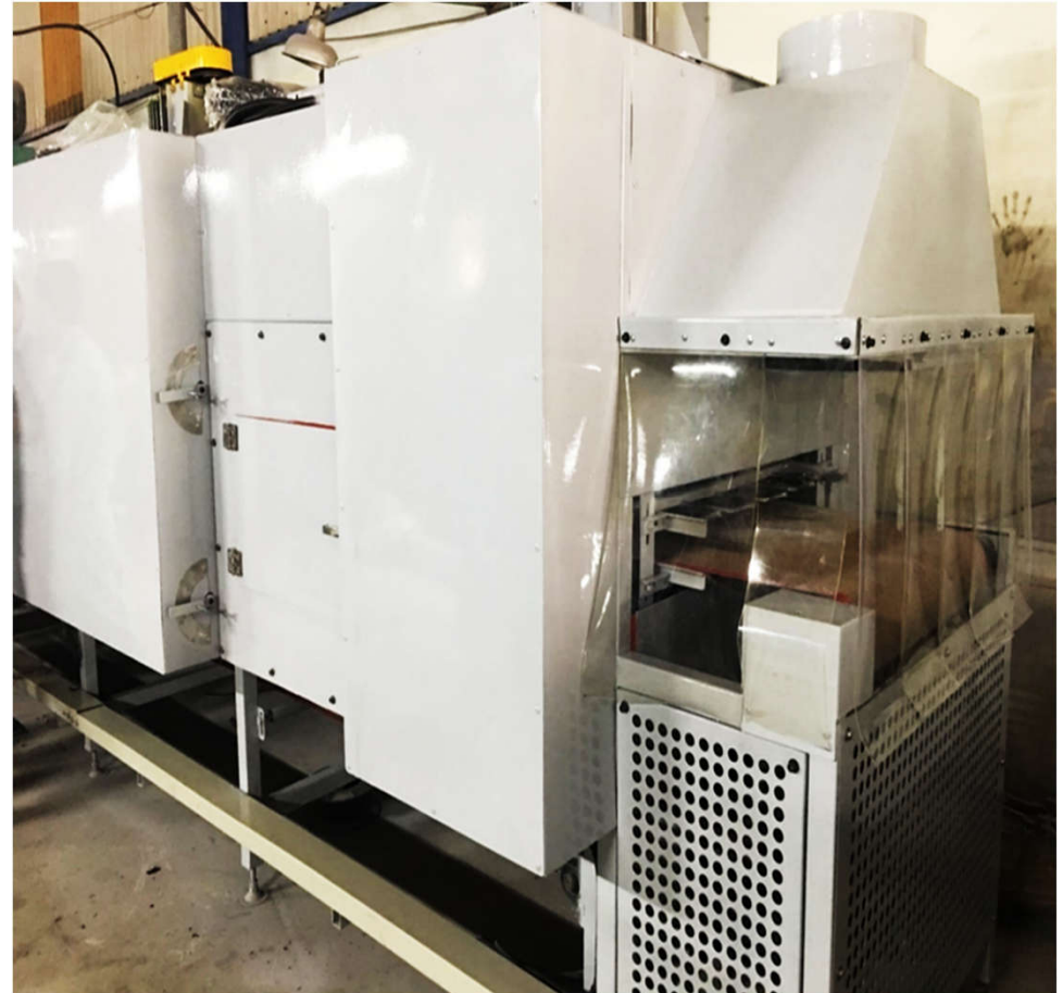
AUTOMATIC FILTER DRYING SYSTEM
